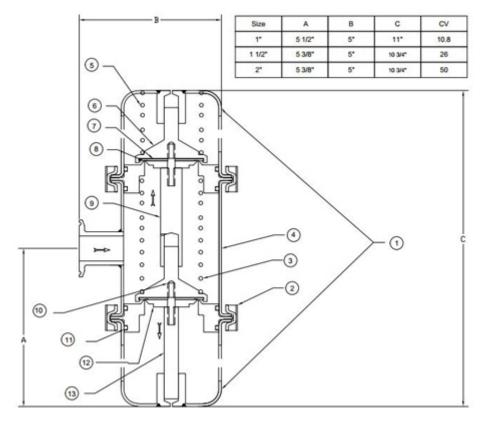
VRV-TC The flow arrow above is shown in the normal flow position When flow reverses, the valve closes
