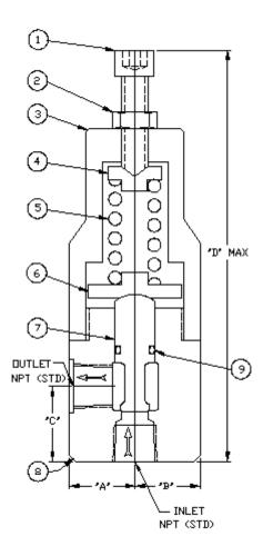
RVC-05-Npt Metal Seated Relef Valve Threaded NPT Connections
